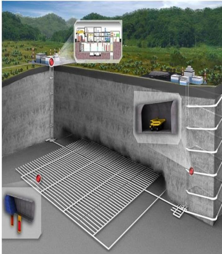
Figure 4 The Korea Reference System for Direct Disposal of Spent Nuclear Fuel
